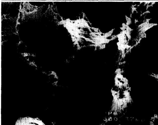
Figure 7 Fractured surface of ethylene-hexene copolymer which exhibited normal behaviour at 80°C under 2.4 MPa
